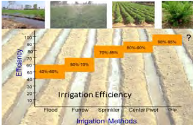
Fig. 5. Irrigation efficiency of different irrigation methods (Courtesy: Rajput, WTC)
