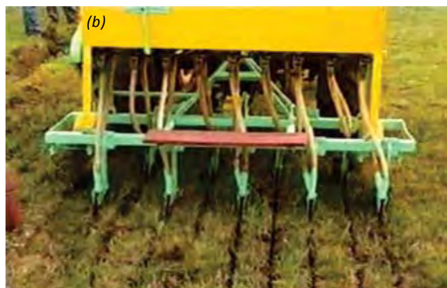
Fig 7. Use of Laser Land Levelling (a) and a Zero-Tillage Machine(b) for Conservation Agriculture
