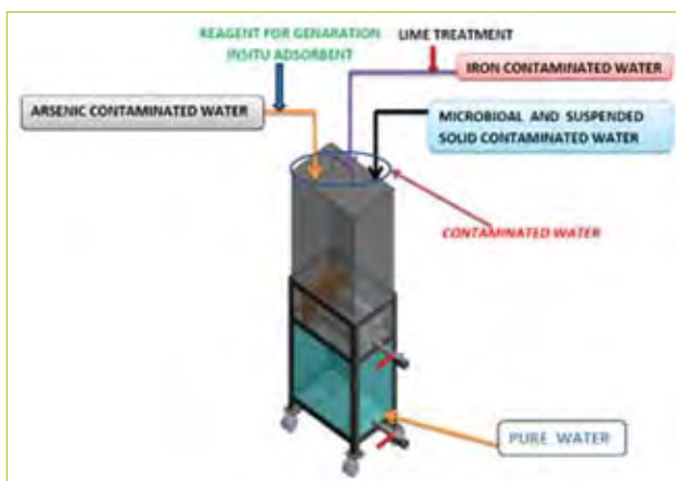
Nanocomposite Ultrafiltration Membrane Device For Domestic Drinking Water Purification W.R.T. Arsenic, Iron And Microbial Contaminations
