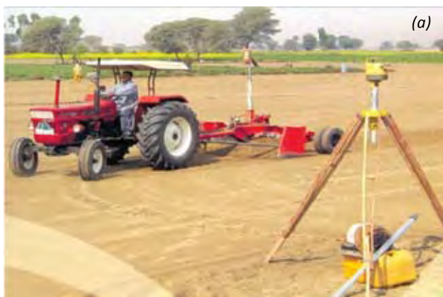
Fig 7. Use of Laser Land Levelling (a) and a Zero-Tillage Machine(b) for Conservation Agriculture
